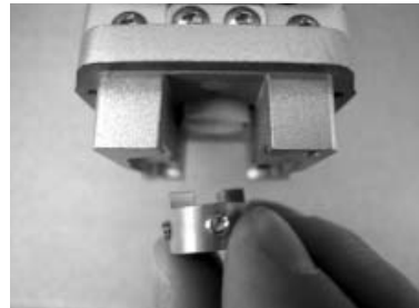
Inserting the coupling (with screws)
